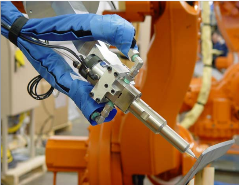
System Integration, Robot Tooling, Dress-Out, Bead-Path Programming and System Run-Off is performed at Sealant Equipment & Engineering
