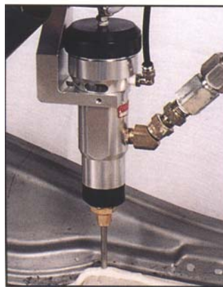
Dispensing Extruded Bead with 2200-033 Snuf-Bak® Valve
